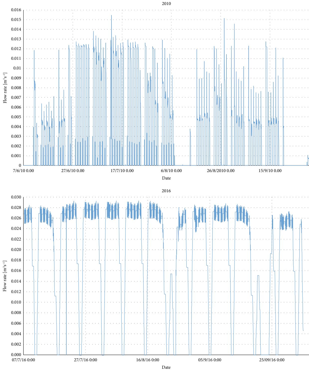
FIGURE 5: Recorded hourly flow rate data [ \text{m}^3 \text{s}^{-1} ] for each monitored season (2010 and 2016).
