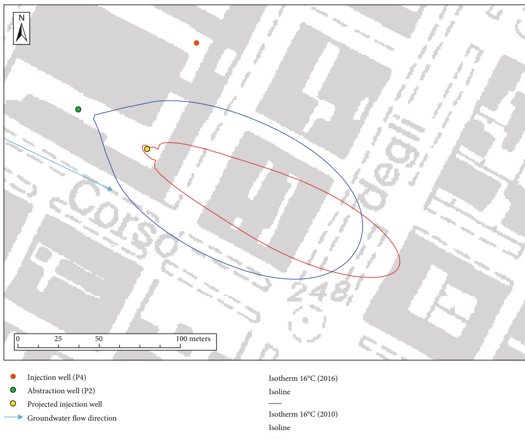
FIGURE 7: Politecnico di Torino open-loop geothermal system thermal affected zone after seasons 2010 and 2016. We highlighted the reinjection well (P4) in the real location and its projection downstream of the abstraction well, along groundwater flow direction.
