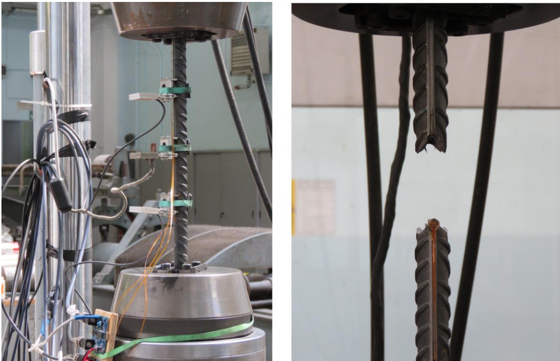
Fig. 12. Monotonic tensile test until rupture of the instrumented bar.
