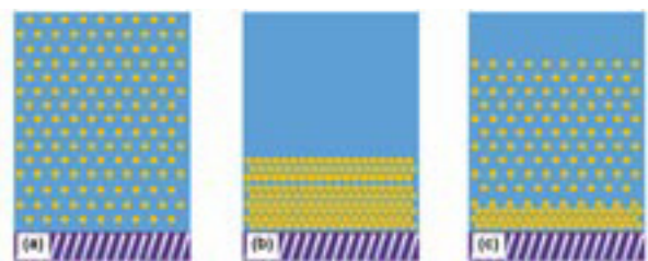
Figure 2: Schematic representation of slurry in systems with (a) no crystal sedimentation prior to filtration, (b) entire crystal sedimentation prior to filtration and (c) partial crystal sedimentation prior to filtration.
