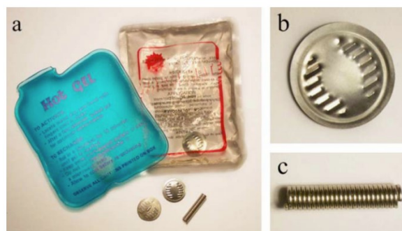
Figure 10. Commercial heat pads (a), with details of flexible disc (b) and spring type (c) triggers. Adapted from [29].
