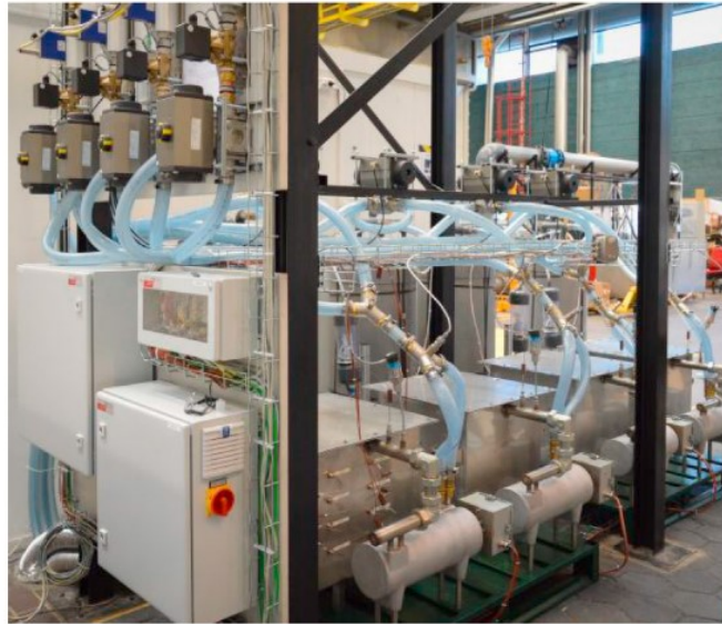
Figure 19. Zeolite based thermochemical system. Adapted from [131].
