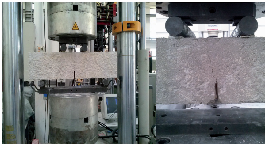
Figure 6 – Four-point bending test, notched specimen.
