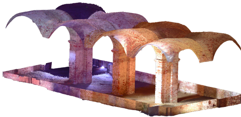
Figure 82. Cleaned point clouds related to the ground, pillars and vaults (perspective view) - (elaboration F. Diara).
