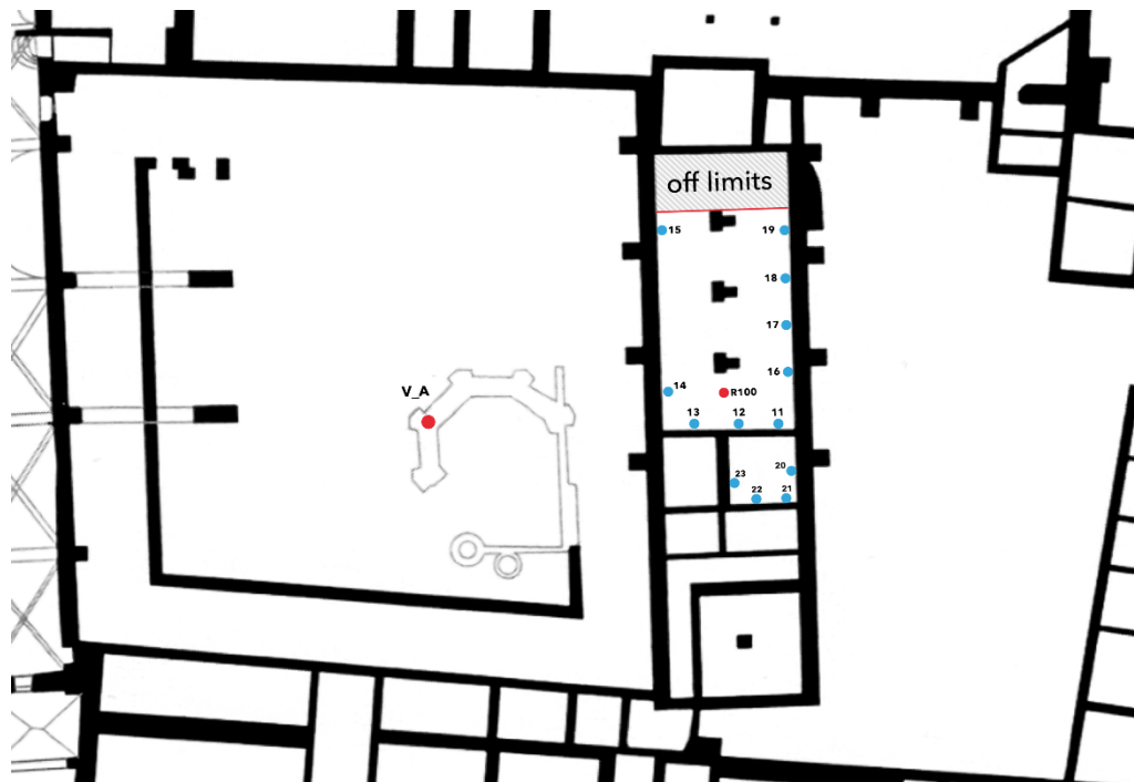
Figure 60. Topographic survey: targets placement, from 11 to 23, inside the refectory
