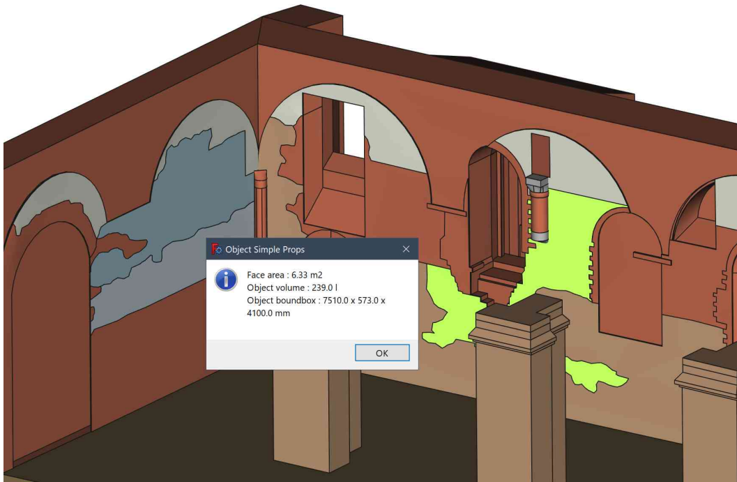
Figure 246. Detail on a stratigraphic masonry unit and its properties on SimpleProperties Macro (elaboration F. Diara).
