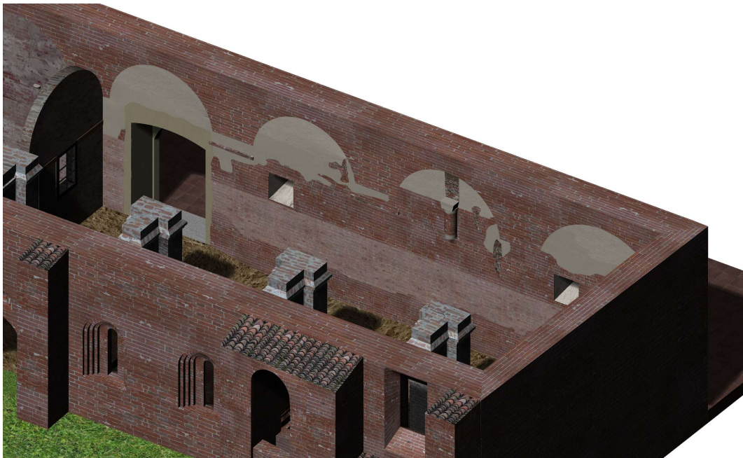
Figure 194. Texturized rendered NURBS model of the refectory. Internal detail of the north wall (isometric view) - (elaboration F. Diara).
