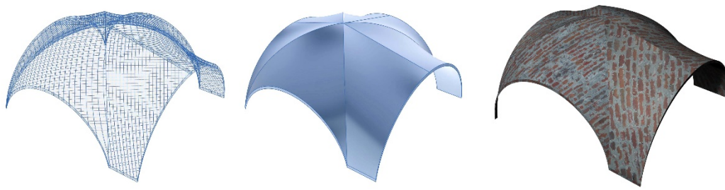
Figure 152. Three different 3D visualization of Rhinoceros. From left: wired; shaded with profiles; render textured view (elaboration F. Diara).
