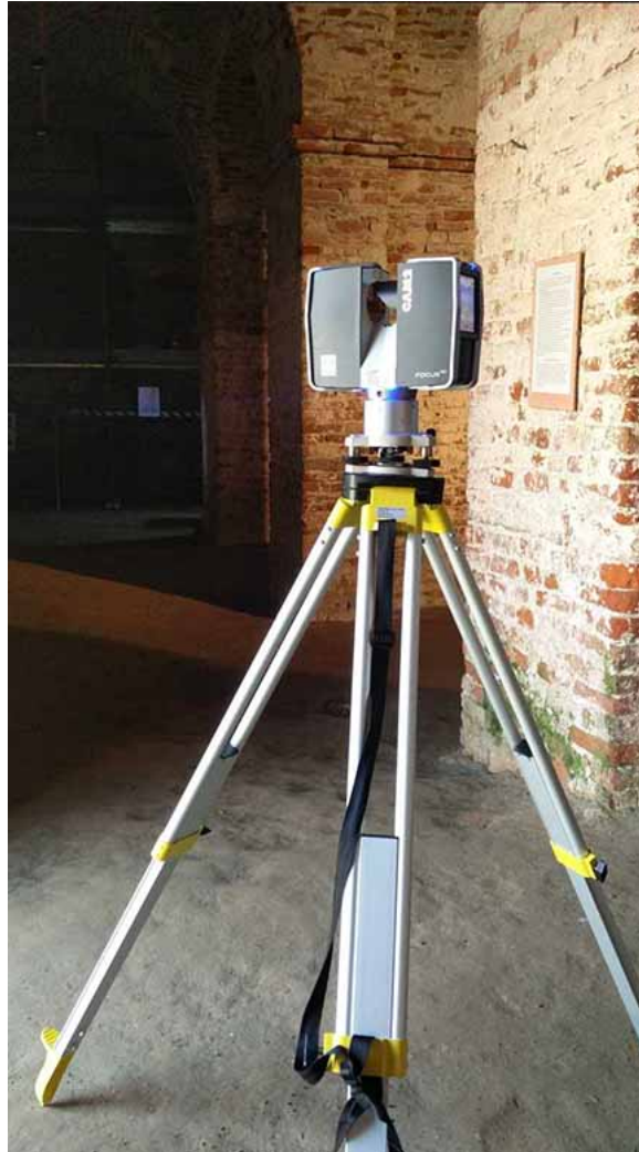
Figure 69. Laser scanner Faro Focus 3D S120 inside the refectory (photo F. Diara)
