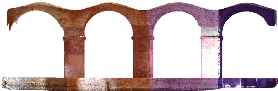
Figure 83. Cleaned point clouds related to the ground, pillars and vaults (X plane view) - (elaboration F. Diara).
