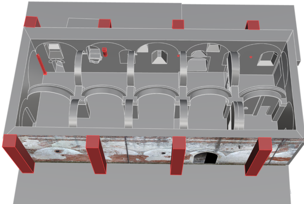
Figure 201. Buttresses, semi-columns and shelves (in red) related to the original ceiling supporting elements. From this reconstruction can be argued correspondences – NURBS model (elaboration F. Diara).
