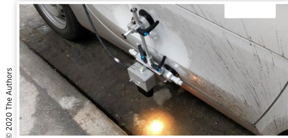
FIGURE 3 Correvit S-Motion on passenger door.
