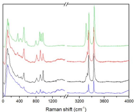
Fig. 3. Raman spectra acquired on coin "6058" (in red, black and blue) and on the clinoatacamite reference sample (in green)
