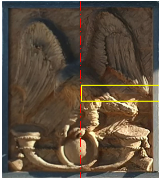
Figure 6. Orthophoto of the eagle's high relief generated using Pix4D (left) and MicMac (right). In the yellow frame it is highlighted an issue with the radiometric equalization of MicMac.
