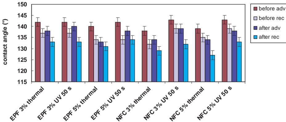
**Figure 3.** Dynamic contact angles of water before and after washing on cotton fabrics finished with Repellan EPF and NFC (adv: advancing; rec: receding) [with kind permission from Springer Science+Business Media: Ferrero F., Periolo M., Udrescu C. Water- and oil-repellent coatings of perfluoro-polyacrylate resins on cotton fibers: UV curing in comparison with thermal polymerization. *Fibers and Polymers* 2012; 13 (2), 191–198, p. 195, Fig. 1].
