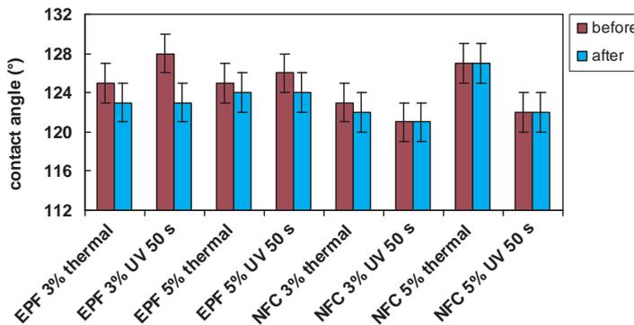
**Figure 4.** Static contact angles of oil before and after washing on cotton fabrics finished with Repellan EPF and NFC. [with kind permission from Springer Science+Business Media: Ferrero F., Periolo M., Udrescu C. Water and oil-repellent coatings of perfluoro-polyacrylate resins on cotton fibers: UV curing in comparison with thermal polymerization. *Fibers and Polymers* 2012; 13(2), 191–198, p. 195, Fig. 2].
