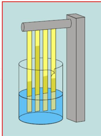
**Figure 1.** Capillary rise method.
