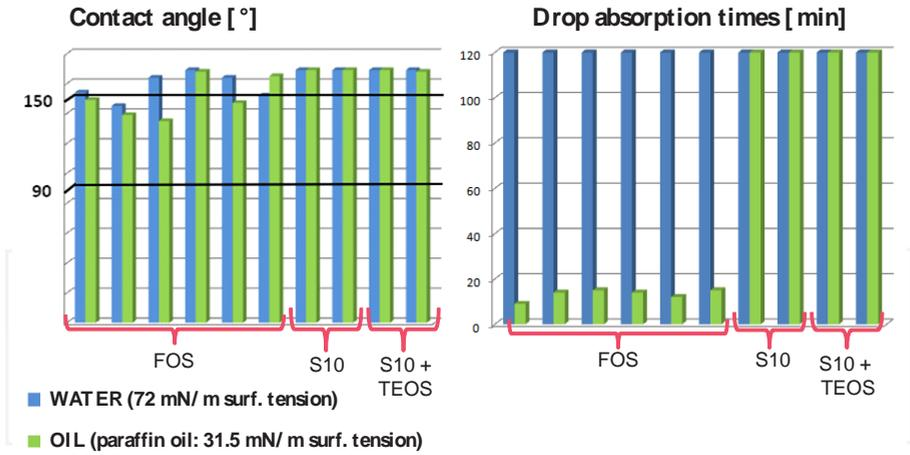
**Figure 7.** Results of contact angle measurements and drop absorption time on cotton fabrics treated with sol-gel finishes. From left to right; for FOS-finished samples add-on and impregnation time: 5% 1 min, 10% 1 min, 5% 2 h, 10% 2 h, 5% 24 h, and 10% 24 h; for the other finishes: 5% 24 h and 10% 24 h.
