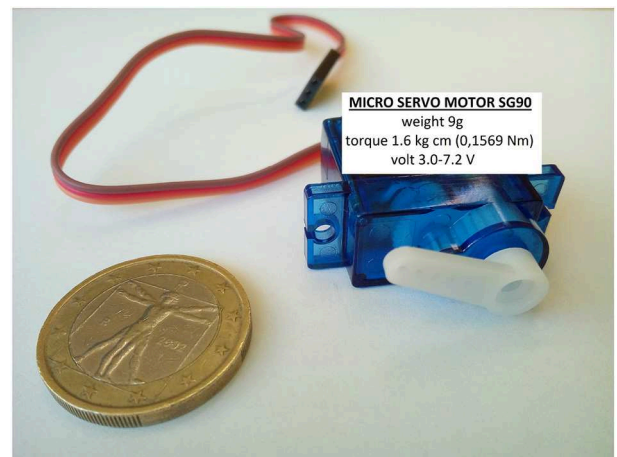
FIGURE 4 | First SG90 servomotor used in our robot.
