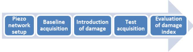
Figure 31: Schematic representation of the experimental procedure.
