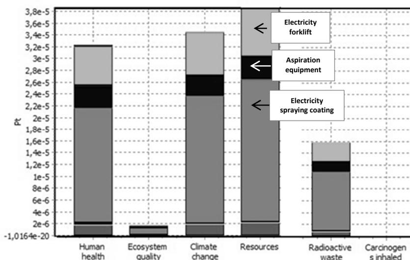
**Figure 3.** Evaluation by impact category of 1 m<sup>2</sup> of nano-TiO<sub>2</sub> coating on travertine.
