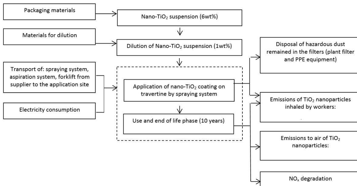
**Figure 1.** Flow chart of nano-TiO<sub>2</sub> coating on travertine.
