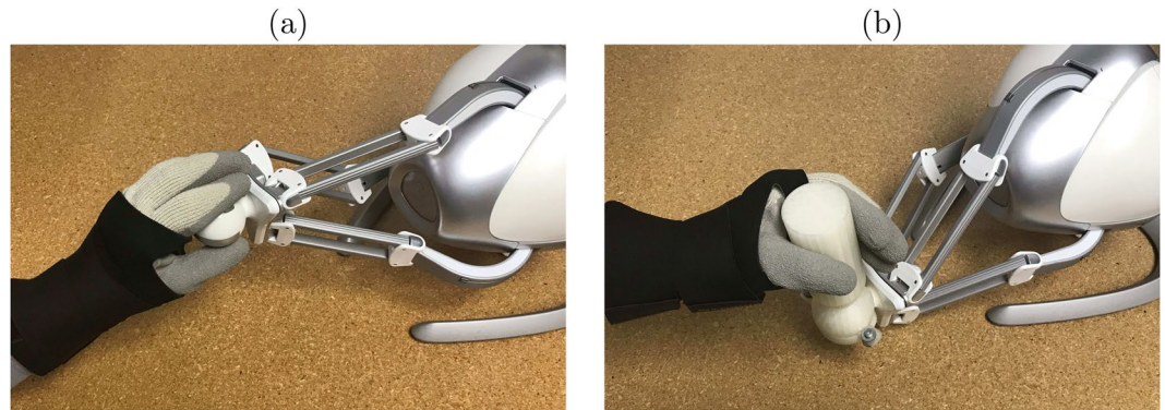
Figure 6. Experimental conditions with the Novint Falcon. Subjects manipulated the end-effector while wearing a thick glove and a wrist brace. They performed the experimental tasks twice, once with the unmodified end-effector (a), and once with the enhanced end-effector (b).
