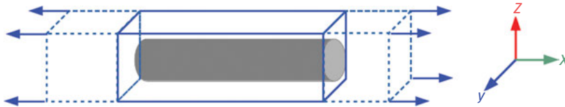
Figure 3.16: Longitudinal deformation of a simulation box.
