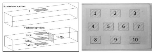
Fig. 2: a) left: areas cut from the specimens to obtain thin sections. b) right: Position of pictures taken from the thin section for image analysis.
