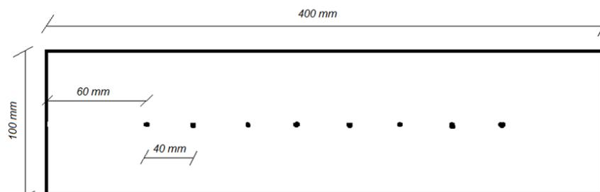
Fig. 6: Laying arrangement for each sample along which to measure the propagation velocity of the ultrasounds by the indirect method.
