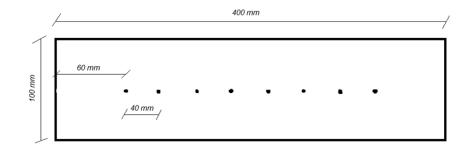
Fig. 6: Laying arrangement for each sample along which to measure the propagation velocity of the ultrasounds by the indirect method.
