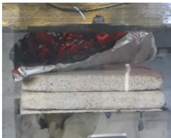
Fig. S9. Capture frame from the video recording the formation of a swollen multicellular carbonaceous layer in the cone calorimetry test for Si-DA2-Mel .
