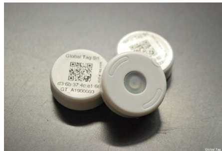
Figure 1: The BLE-sensor (15 mm radius) is able to communicate via Bluetooth with the receiver, generally a smartphone. It gives information of temperature and humidity and is supplied by a CR2032 coin battery. Image taken from: https://www.global-tag.com
