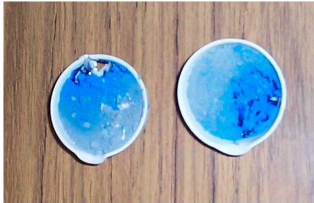
Figure 3. Thermal runaway occurring in samples processed in multi-mode applicators, at 2.45 GHz, for power density exceeding 60 W/g.
