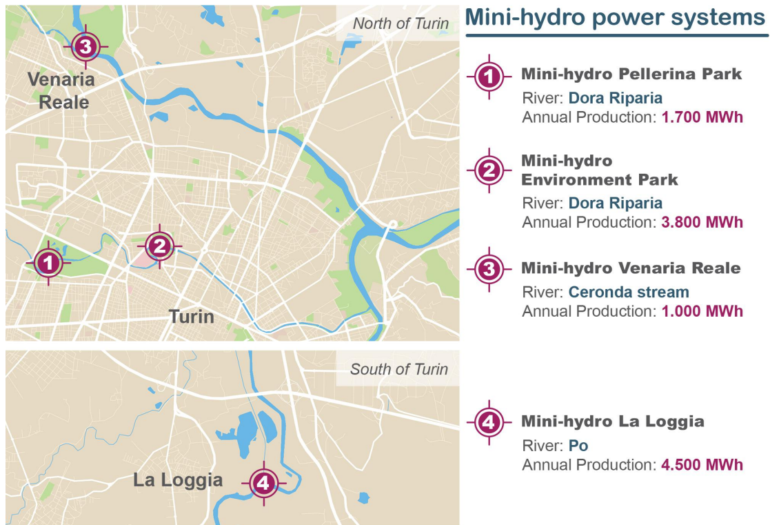
Fig. 4. Distribution of mini-hydro power systems in the urban and suburban area of Turin.
