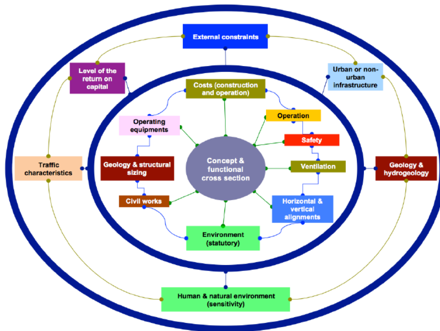
Figure 1.1 Road tunnel as a complex system (PIARC) [1]
