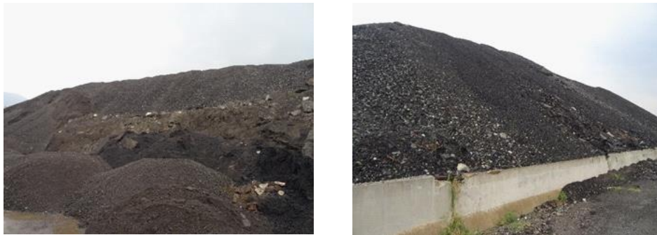
Figure 2.6 Large piles RAP visible in production plants (SITALFA plant )
