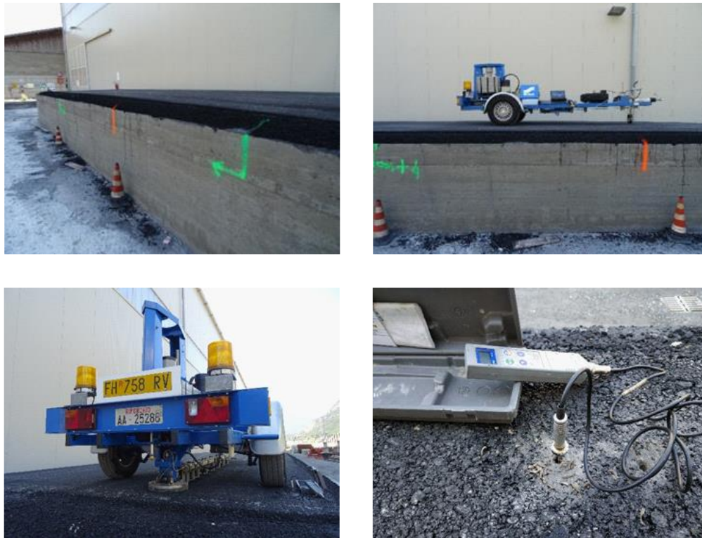
Figure 5.11 FWD testing over the full scale trial section
