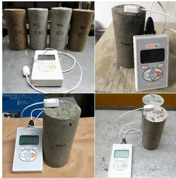
Figure 3.8 Thermal conductivity measurements
