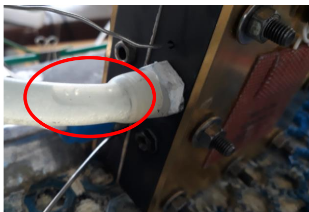
Figure 6.10. Crossover effect (red circle) produce by O 2 backpressure increment from 0.5 to 1bar.
