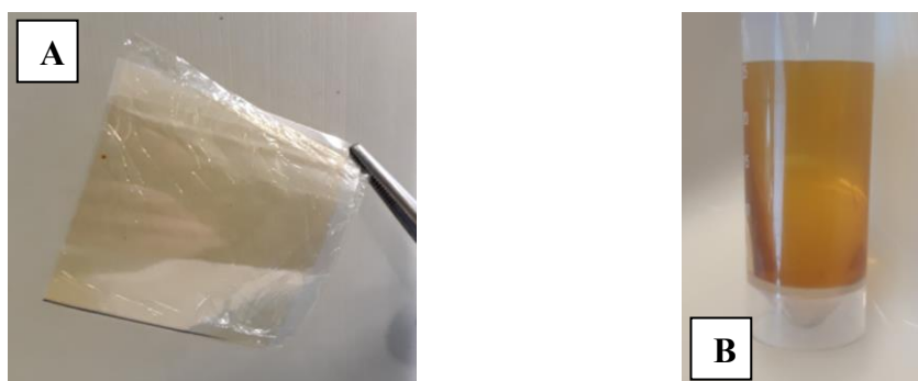
Figure 2.1 A) FAA-3-50 membrane in dry form. B) PBI Dopozol membrane during the activation in KOH 6 M solution.
