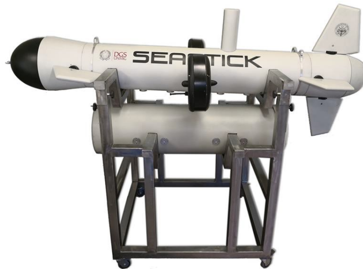
Figure 50. Autonomous Underwater Vehicle equipped with a miniaturized laboratory, developed by Politecnico di Torino, for autonomous heavy metal detection in seawater near offshore hydrocarbon platforms.
