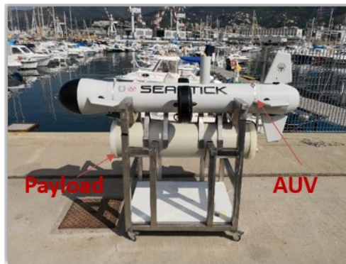
Figure 83. AUV - Payload prepared for first test on field.
