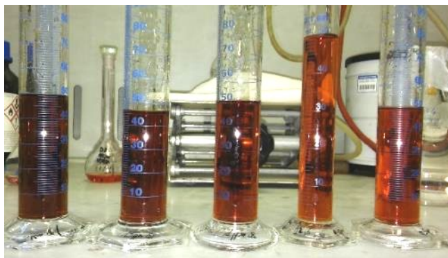
Figure 30. Complexed samples at pH 4, From the right 0.1 – 0.25 – 0.5 – 1 – 2 ppm
