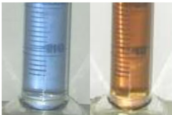
Figure 27. Solution containing 1 ppm of Zn(II) complexed with Zincon. On the left the reaction occurs in buffered condition (pH 9). On the right a basic condition.
