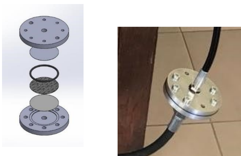
Figure 63. Filter support CAD design (left) and manufacturing (right).
