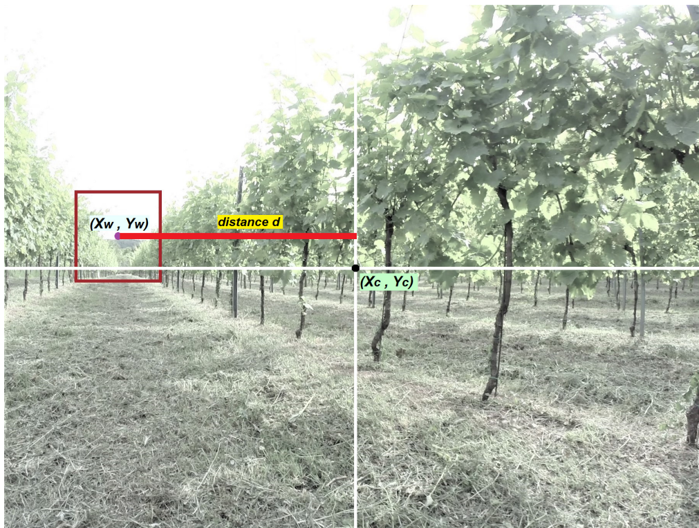
Figure 2. Depth-map algorithm scheme. The end of the vineyard row detected is represented by the red rectangle. The value d , on which the control algorithm is based on, is computed as the horizontal distance between the center of the camera frame and the center of the detected window.
