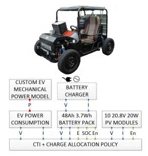
**FIGURE 9.** The custom EV: picture (top) and energy subsystem modeled with the proposed framework (bottom).
