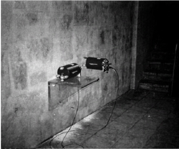
Fig. (6). Seismometers respectively fixed to a cantilever and the wall along two orthogonal directions.
