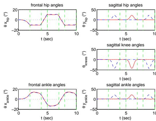
Figure 27. Step Machine—Joint angles (dashed line = left leg).
