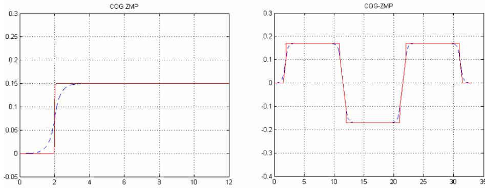
**Figure 7.** (left) sagittal plane  $COG_{prev}$  (dashed) and  $ZMP_{prev}$  in the extreme of equilibrium exercise and (right) Frontal plane  $COG_{prev}$  (dashed) and  $ZMP_{prev}$  in the step machine exercise.
