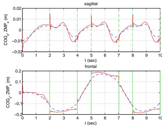
Figure 26. Step machine—Coordinate behavior ZMP and COG (dashed).
