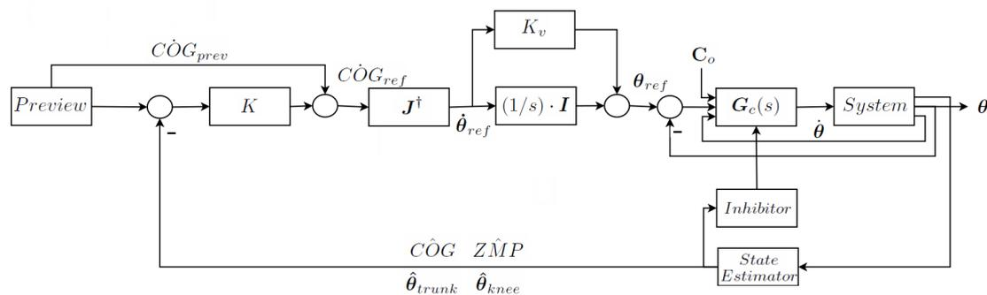
Figure 8. The postural control loop—one for each plane.
