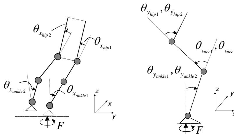
Figure 2. The exoskeleton: frontal and sagittal planes.
