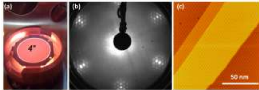
Figure VII.4. (a) 800 °C hot 4 inch wafer in the growth chamber. (b) Low energy electron diffraction (LEED) pattern of h-BN/Rh(111) at 60 eV kinetic energy. (c) STM image of the same surface with U_t = -1.2 V and I_t = 0.5 nA.
