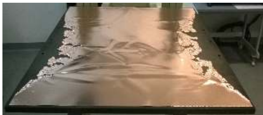
Figure V.6. Higher T near the edges of the substrate causes local Cu melting while the inner part is unaffected.
