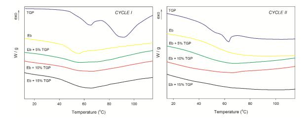
Figure S5. DSC curves ( $1^{st}$  and  $2^{nd}$  run) for E0, TGP and EP samples at a heating rate of  $10^{\circ}$ C/min.
