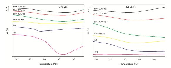
Figure S4. DSC curves (1st and 2nd heating runs) for E0, tea and ET samples at a heating rate of 10°C/min.
