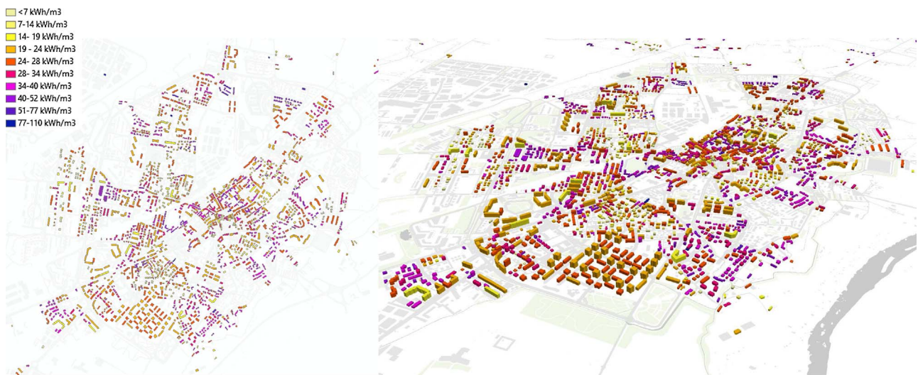
Fig. 10. Urban Energy Map (2D and 3D); energy consumption for space heating (kWh/m³/y).
