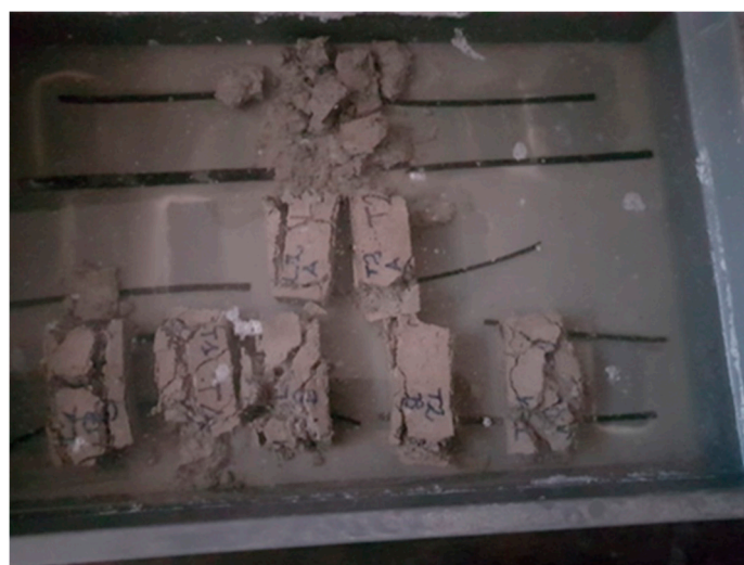
Figure 12. Imbibition of L1, L2, T1 and T2 specimens after salt crystallisation cycle and flexural strength test. Specimens breakdown.
