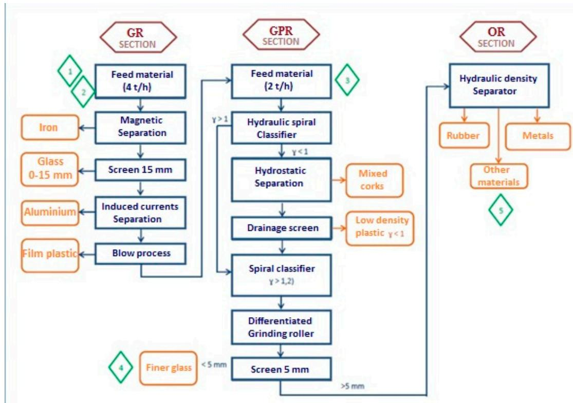
**Figure 2.** Plant operation for the recovery of glass waste<sup>3</sup>: brown indicates the main section of the plant.
