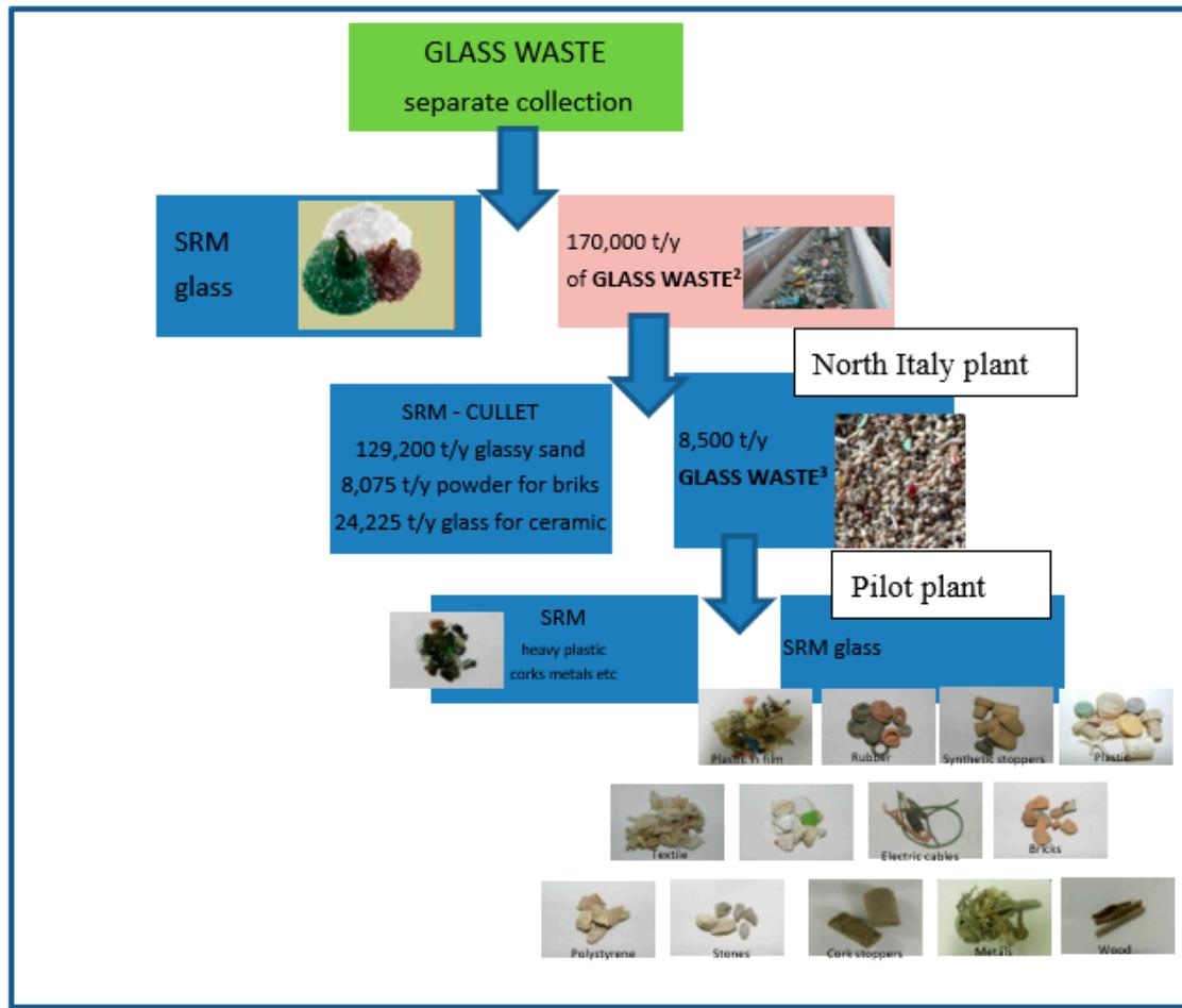
**Figure 1.** Flowsheet of production of glass waste<sup>3</sup> treated in the North Italy pilot plant.
