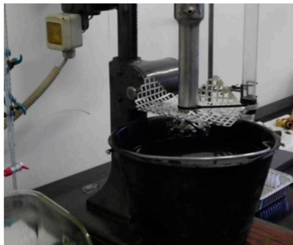
**Figure 3.** The bath extractor separator.
