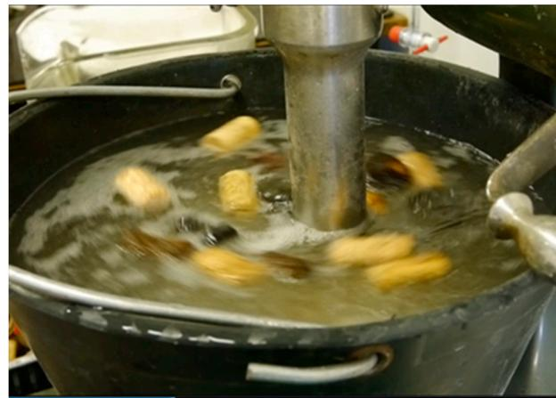
**Figure 5.** The bath extractor separator as a product of separation with stoppers (cork and synthetic).
