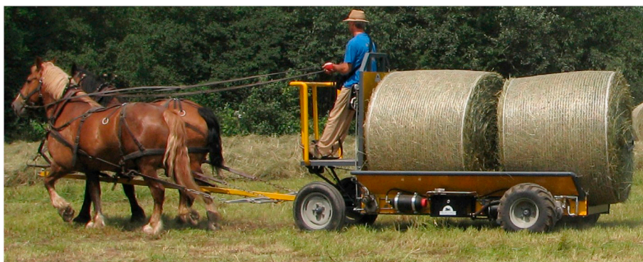
Fig. 8. Hydraulic round bale loader (Courtesy of EQUI idea).
