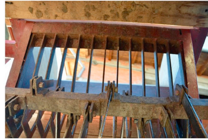
Fig. 5. Self-produced chestnut deburring machine.
