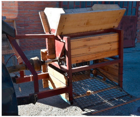
Fig. 5. Self-produced chestnut deburring machine.
