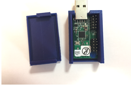
Figure 4: Example of a small USB receiver suitable for operations in the absence of power supply. The dimensions are 3\text{ cm} \times 4.5\text{ cm}
