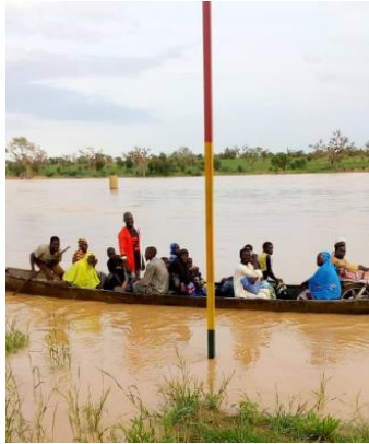
Figure 7. Colored hydrometric staff at Garbey Kourou, Niger.
