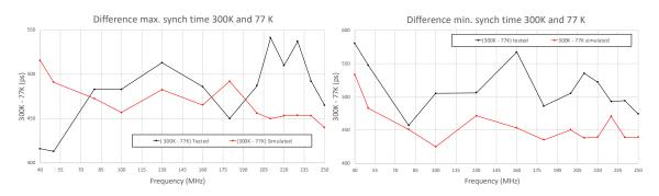
**Figure 8**. Results of synchronisation module expressed as time difference (300 K - 77 K), for both minimum and maximum time delay. In the graph are reported also time delay obtained from test and SPICE simulation.
