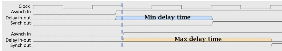
**Figure 6.** Synchronisation time diagram. If the input signal occurs immediately before the falling edge of the clock, the synchronisation lasts for 1 clock period and half, otherwise it lasts for 2 clock periods and half.
