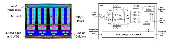
Figure 1. On the left the layout architecture of ALCOR, on the right the schematic diagram of the single pixel.
