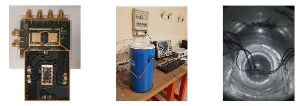
**Figure 7**. From left: The Test Chip is wire bonded in the center of the test board; Test setup used to measure time delays; Test board is dipped inside the small dewer in a bath of liquid Nitrogen at 77 *K*.
