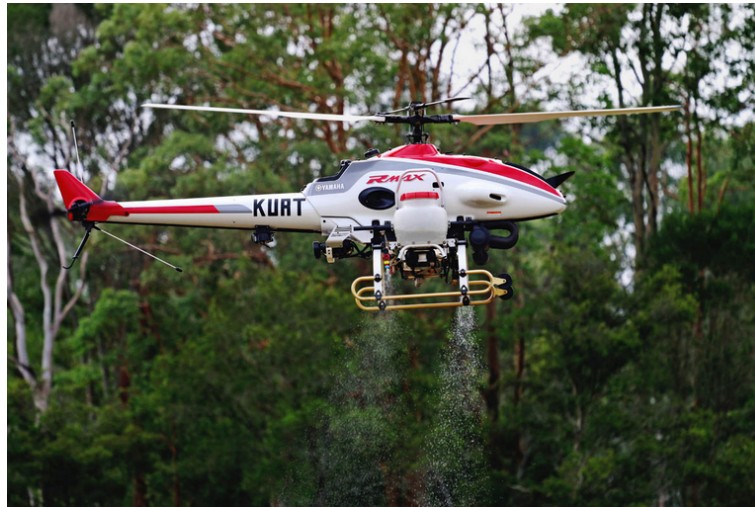
Fig. 2.2 RMAX, a very popular drone which has been utilized for many years in agricultural applications. Reproduced from [14].
