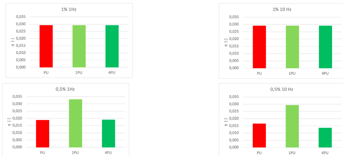
Fig. 6. Loss factor in different strain and frequency conditions for different number of PU coating layers.
