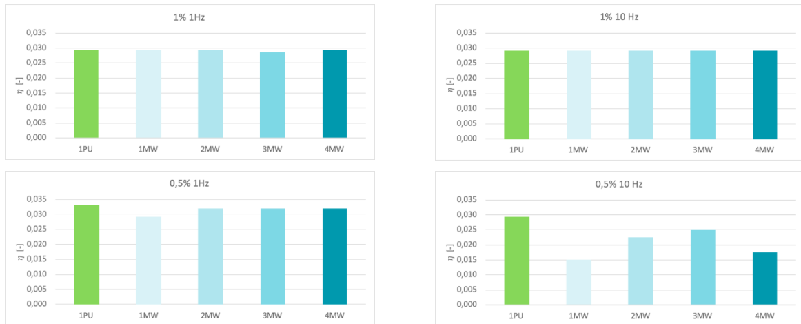
Fig. 7. Loss factor in different strain and frequency conditions for different number of CNT coating layers.
