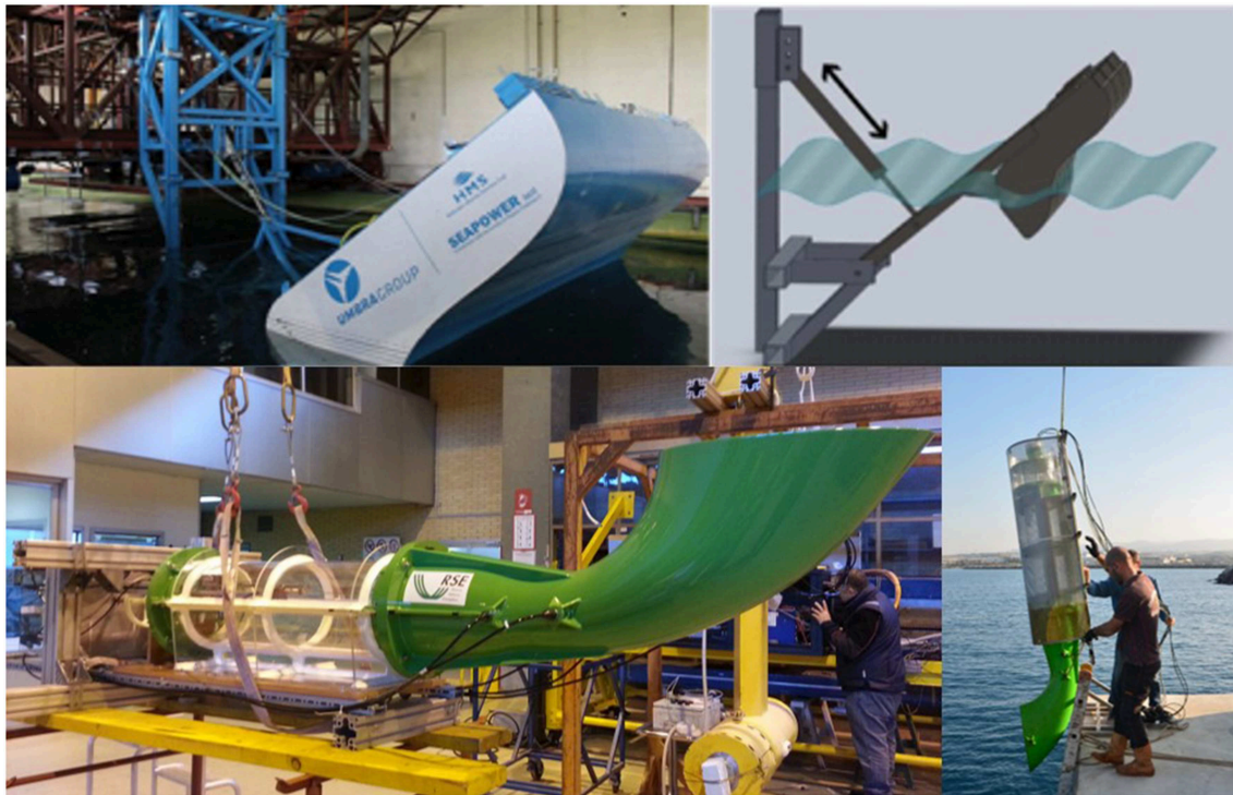
FIGURE 8 | (Top) Full scale GEL prototype (Left) and schematic representation of GEL (Right). (Bottom) Full scale WAVESAX prototype (Left) and its deployment in Civitavecchia (Right).
