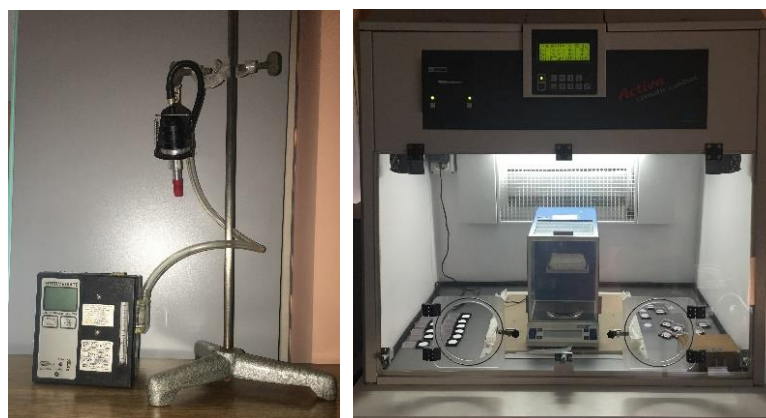
Figure 12 Personal sampling line (left), analytical scale in the climatic cabinet (right)
