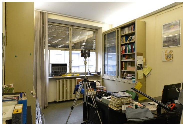
Figure 20 CAM2 Focus 3D laser scanner
