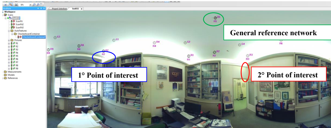
Figure 21 3D Base model of the test area, reference system, and points of interest location
