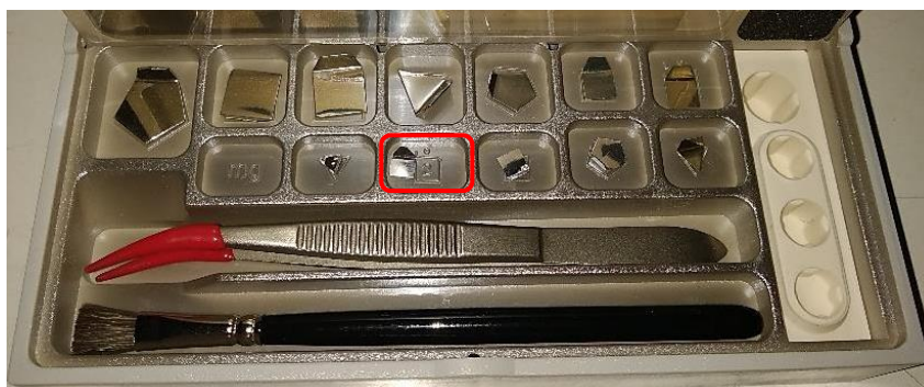
Figure 13 Class E1 set of reference masses, compliant with ISO 15767:2009 standard - the red box indicates the two-milligrams mass used
