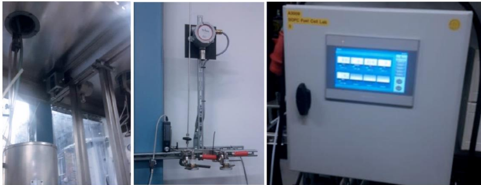
Gas sensors inside the setup and on the cooling devices – control system
