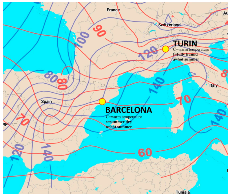
Figure 1. European heating index (EHI) in red lines and the European cooling index (ECI) in blue lines (source: authors' elaboration from References [62,63]).
