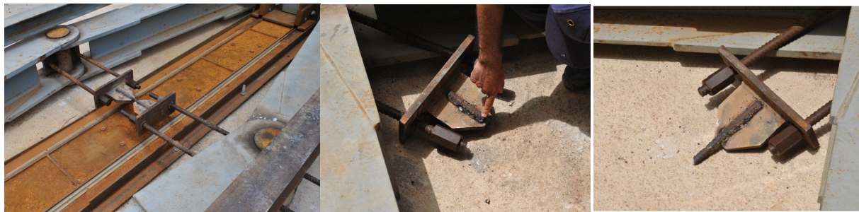
Figure 7: Fuse device before and after failure.
