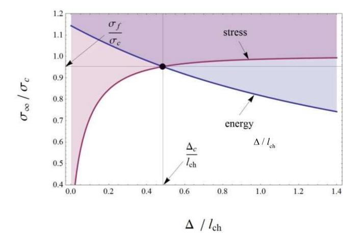
Figure 3. Admissible failure stresses vs. finite crack increment according to discrete energy balance and stress requirement for  $a=0.6\ l_{\rm ch}$ . The actual failure stress is the minimum among admissible values.
