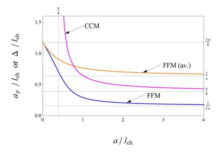
Figure 4. Finite crack increment according to FFM approaches and process zone size at incipient failure according to CCM vs. crack radius.
