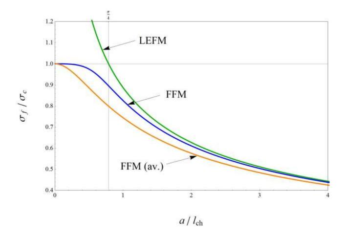
Figure 8. Failure stress vs. crack radius according to FFM coupled with point-wise and average stress conditions.
