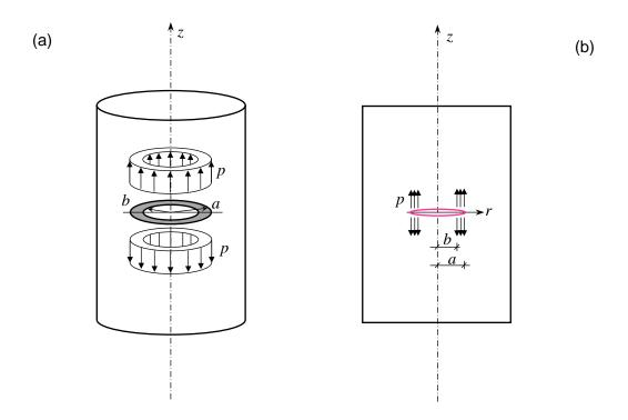
Figure 2. Penny-shaped crack under annular constant stresses: 3D view (a); longitudinal section (b).
