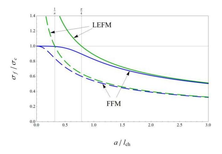
Figure 9. Failure stress for a solid containing a penny-shaped crack (continuous line) and for a slab containing a through-thickness crack (dashed line) vs. crack radius/half-length according to FFM and LEFM.
