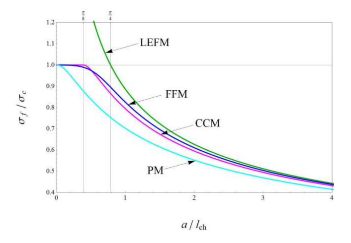
Figure 5. Failure stress according to FFM, LEFM, PM and CCM vs. crack radius.
