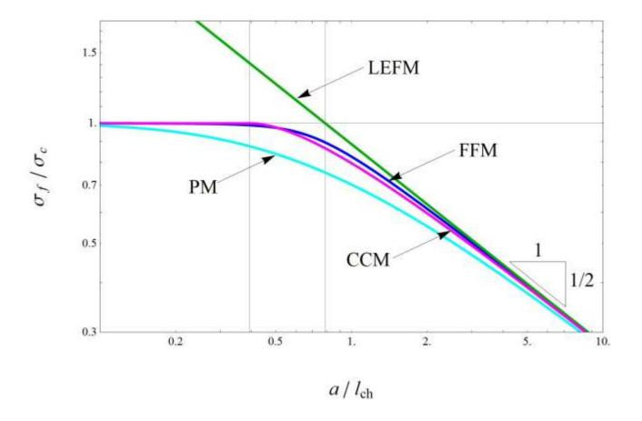
Figure 6. Failure stress according to FFM, LEFM, PM and CCM vs. crack radius (bi-logarithmic plot).
