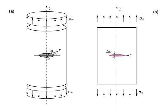
Figure 1. Penny-shaped crack under uniform remote stress: 3D view (a); longitudinal section (b).
