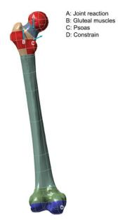
Fig. (1). Load and boundary conditions related to gait heel strike phase.
