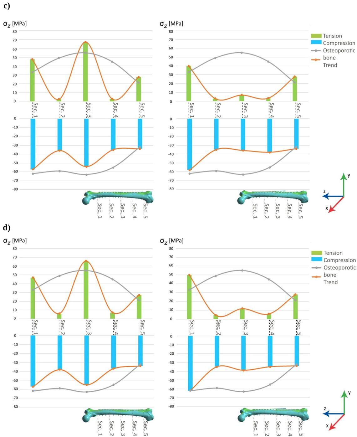
**Fig. (3).** Average tension (green) and compression (blue) longitudinal stress components  $\sigma_z$  for not fractured femur, both in the unplated (grey) and in kissing and overlapped plates configurations (stainless steel (a, c) and titanium alloy (b, d), healthy (a, b) and osteoporotic bone (c, d) during heel-strike phase, in the five cross sections chosen. The orange lines highlight the stresses trend along the diaphyseal axis of the femur in the different configurations.
