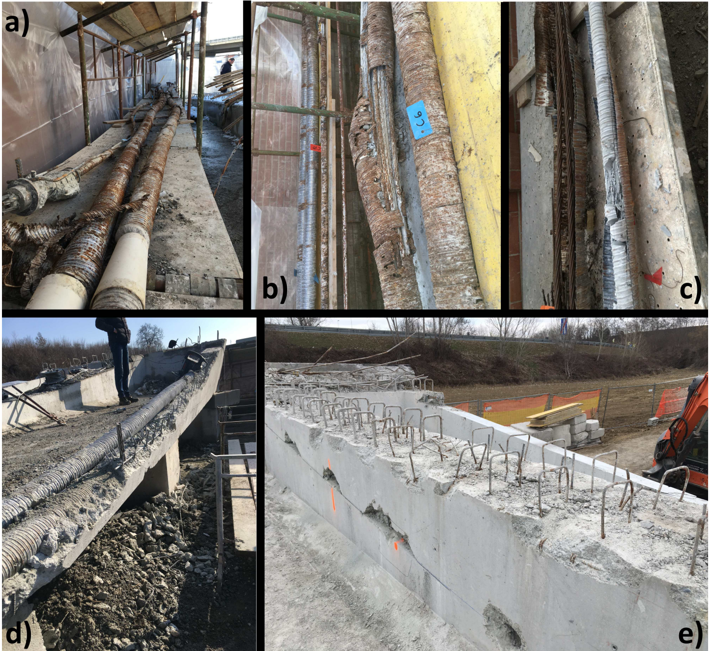
Figure 3: a,b) oxidated cables. c) in situ casted cable. d) dissection and extraction of one of the main cables. e) extracted stirrups
