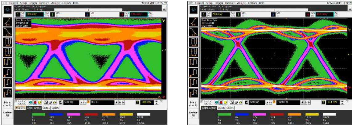
Figure 15: Asymmetric eye diagrams for one of the pilot modules before (left) and after (right) QPLL installation. The amount of jitter decreased significantly after QPLL installation.
