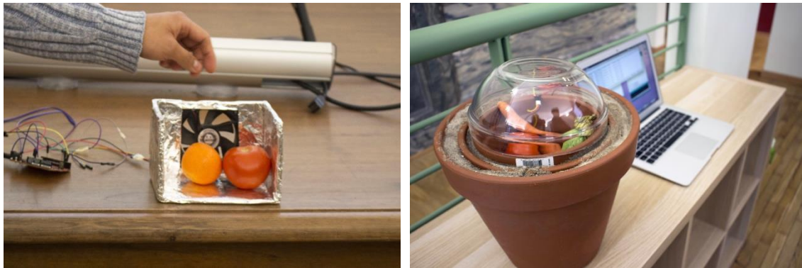
Figure 4: Temperature and humidity monitoring prototypes
