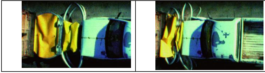
Figure 30 - Truck mounted attenuator. and crash test results
