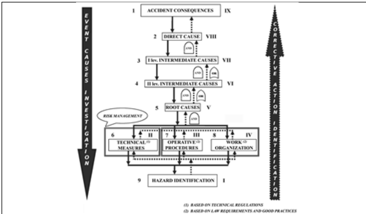
Figure 4 - home screen of the CCCP software (above) and flow chart of the accidents analysis two-way approach (below).
