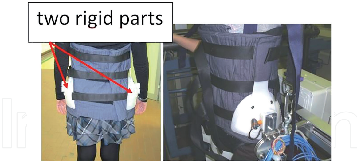
Figure 13. Textile corset, used to connect the patient to P.I.G.R.O.
