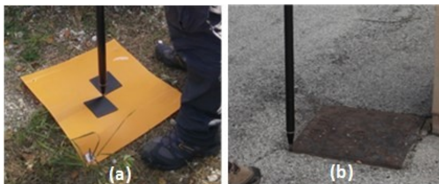
Figure 3. fabricated GCP markers (a), surveyed natural formations (b) [1].
