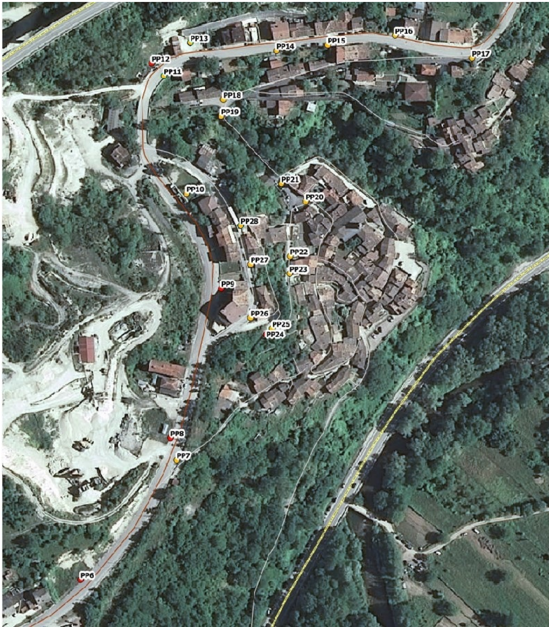
Figure 4. Locations of the 23 GCPs throughout Pescara del Tronto (red denote fabricated GCP markers, and yellow markers denote natural formation GCP markers [1]).
