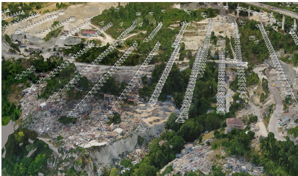
Figure 10. Industry standard mission plan: camera locations and angles represented as triangular prisms.
